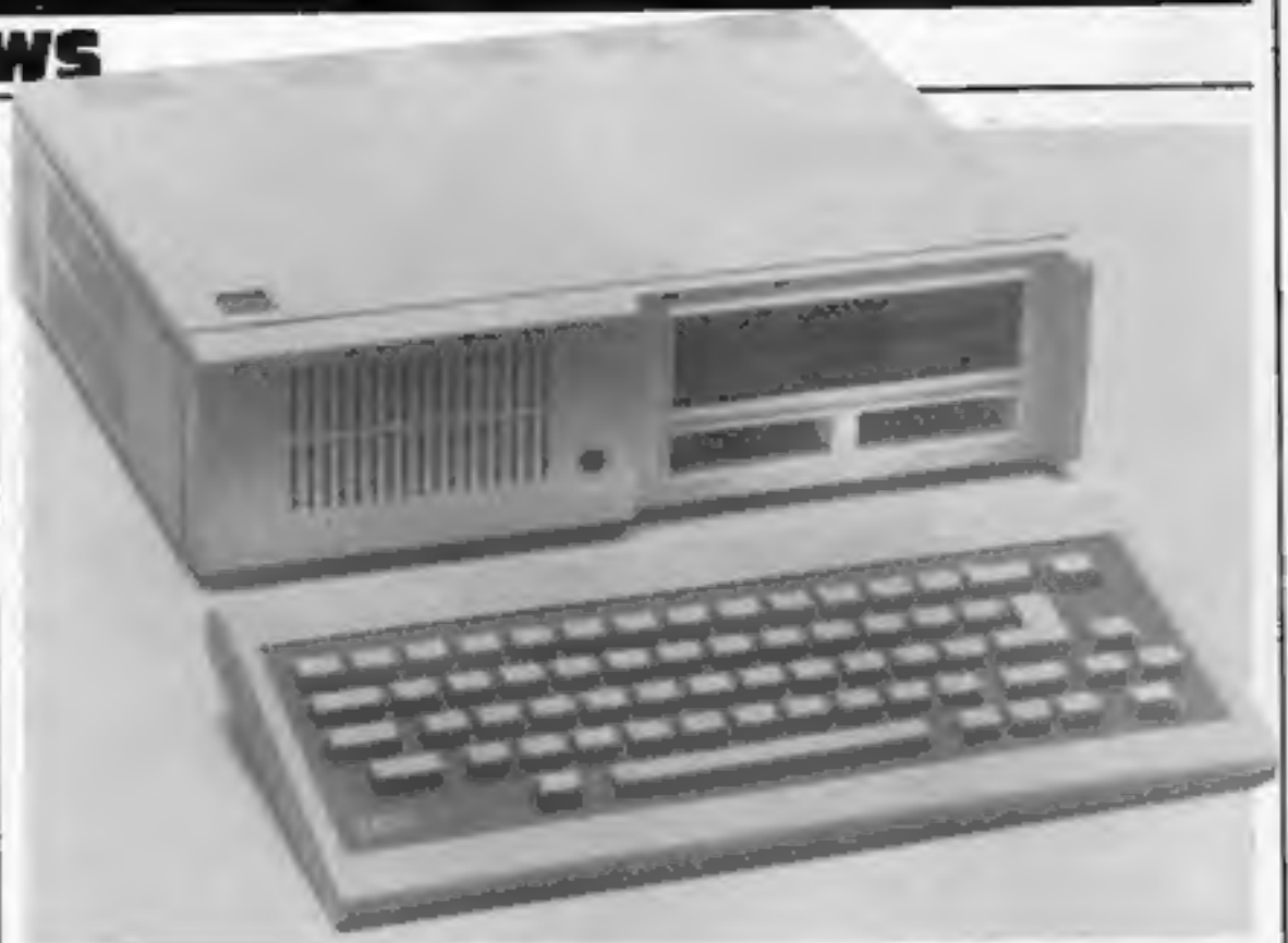
Both models of the Junior look the same, but in the cheaper version a blanking plate covers the opening for the disc drive. Below it are two cartridge slots. The round opening is for the infra red control and the grille is for the speaker and for ventilation
